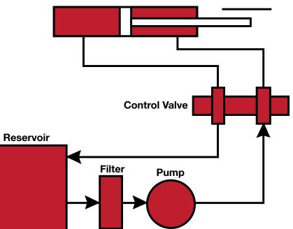
Although systems are extremely power-dense, hydraulic actuators have the lowest energy conversion efficiency of the three actuator types. (Source: Exlar) 40 percent globally. Furthermore, the studies indicate that 40 percent of industrial applications do not use energy-efficient technologies, intensifying the energy consumption issue. Transportation consumes more than 25 percent of US electrical power.
